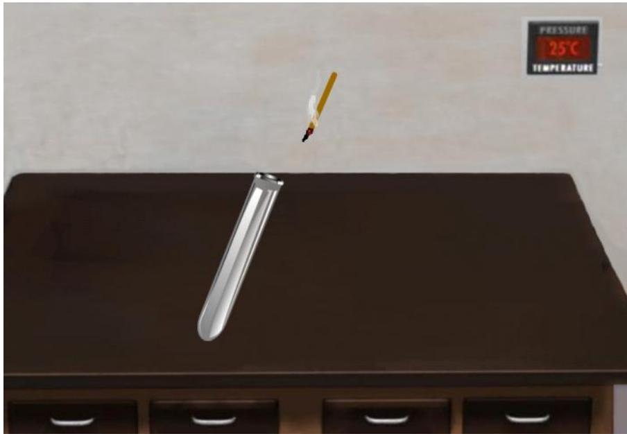
Optional - test the gas - this time place the flame into the gas in the test tube. (it should go out)
