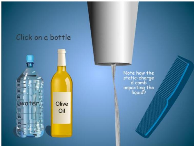
Here we have a lab set up in which we are going to test water and oil's behavior around a static charge. We can build up a static charge with a balloon or a plastic comb rubbed against clean dry hair. The comb will give many electrons to your hair leaving the comb to be more positively charged than is normal.
