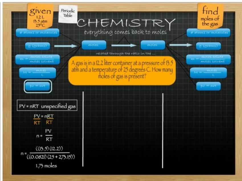
Let's try an example. A gas is in a 12.2 liter container at a pressure of 13.5 atm and a temperature of 25.0 degrees Celsius. How many moles of a gas is present?
